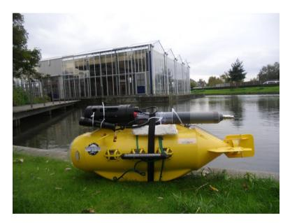
Figure 4 Underwater drone equipped with water quality sensors (multi-parameter probe on top and CTD on the side) and with HD video cameras (at the front).
